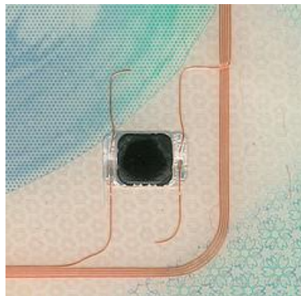
Figure 1: Directly visible contactless chip and antenna in UK passports
